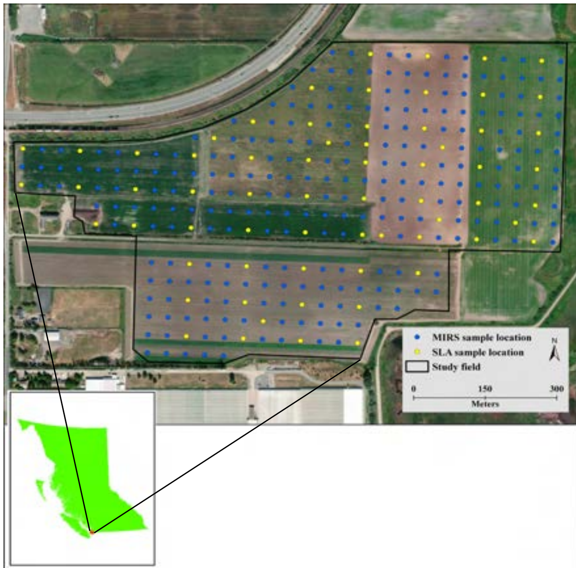
Fig. 2. Location of the study site (49.08 N, 123.06 W) showing the standard laboratory analysis (SLA, n = 62 ) and mid-infrared spectroscopy (MIRS, n = 308 ) sample points following a 40 \times 40 m grid. The SLA samples were also analyzed with MIRS.
